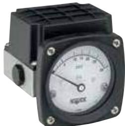
4-20 mA transmitter in NEMA 4x IP65 plastic enclosure with terminal strip (1/2" female NPT conduit connection)
