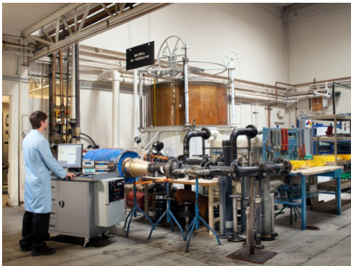
Primary standard 100 cubic foot bell prover capable of producing flow rates from 0.00035...1000 scfm (0.01...28,317 slpm).
