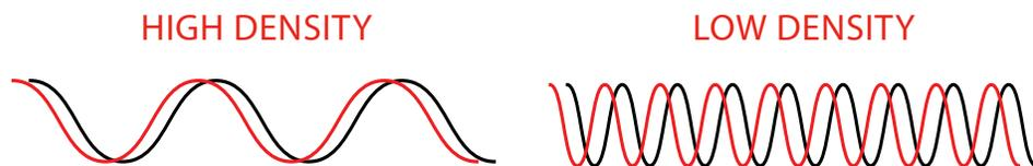
RCT1000 Coriolis mass flow meters operate at low frequencies which reduce the formation of air slugs in liquids with entrained air. This operation keeps liquids more homogeneous and provides less erratic readings.
